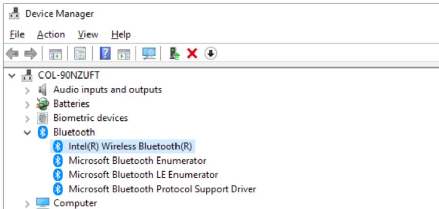
*Note: the name(s) of the internal Bluetooth device(s) will differ from computer to computer. Generally speaking, you should disable all Bluetooth devices which do not contain the text "Microsoft Bluetooth" or "TDK Bluetooth".*
